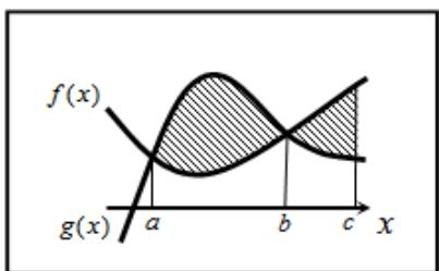
$$\begin{aligned} S_1 &= \int_a^b (g(x) - f(x)) dx \\ S_2 &= \int_b^c (f(x) - g(x)) dx \\ S &= S_1 + S_2 \end{aligned}$$
